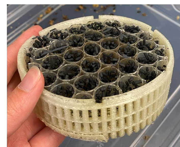
CCF inside of a 3D printed mold after coffee smoke has passed through the filter
